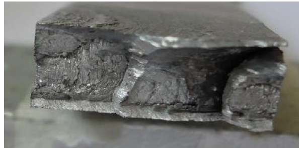
Figure 4. Fracture cross-section of the air welded sample
