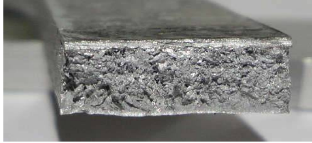
Figure 3. Fracture cross-section of the welded sample underwater
